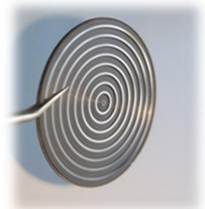
Fig. 1 The photo of thin silicon-based phase shifting element for the 0.6 THz
